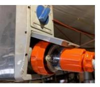
Adjust back bar • locking levers as per user's requirement. **Back bar locking** levers can be tightened, to adjust the height of the rotating blade.
