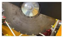
Check the rotating blade alignment.
